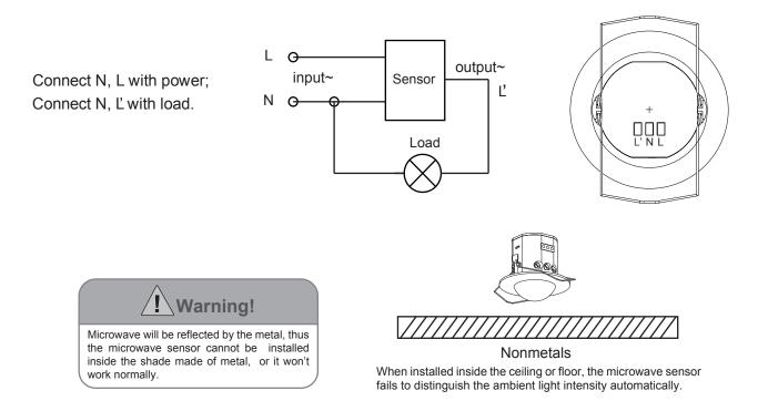
You can install one or more inside the ceiling or floor to control the whole passageway.
