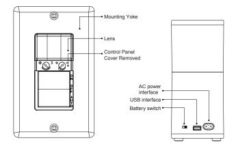
Note: Battery switch is closed when the product is out of the factory. When it is first used, please turn on the power switch.
